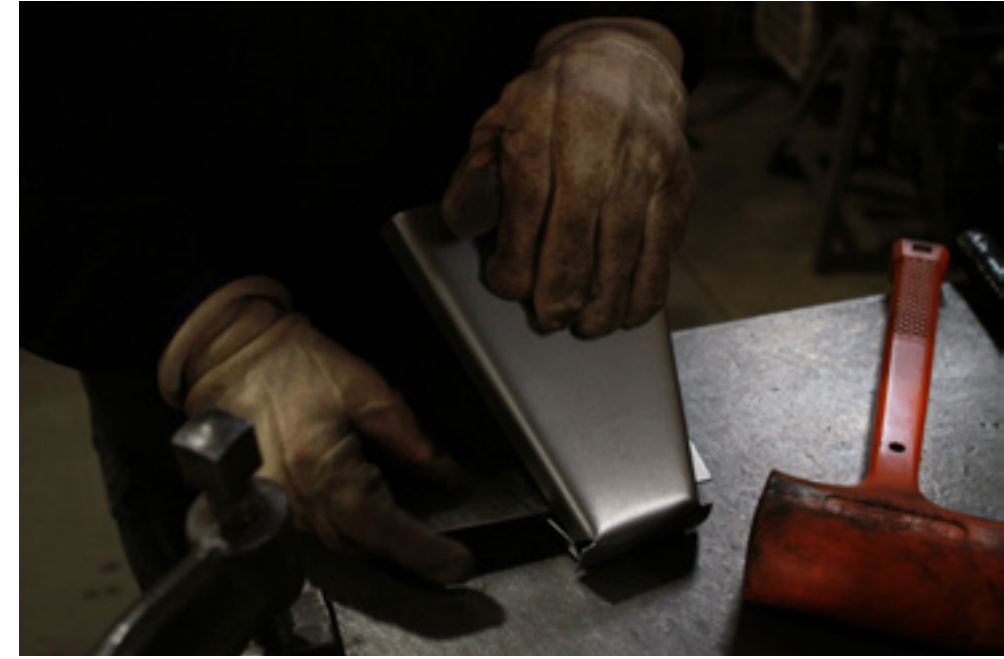
The cowbell is bent into its bell shape by hand. A mallet is then used to make sure the edges of the bell align perfectly.
