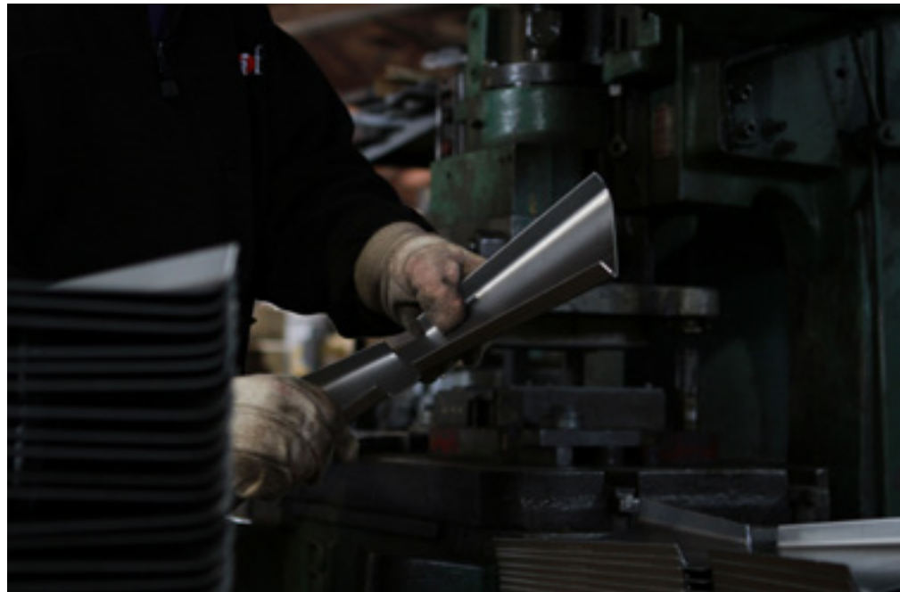
The steel is cut again, this time into an hour-glass shape. The edges are then crimped in a press.
